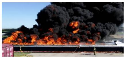
LASTFIRE has carried out the most comprehensive series of end-user driven foam application tests for more than 40 years including different application methods, different fuels and different foams. Largest test fire – 40m foam flow!
